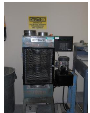
This machine subjects each sample to a pressure stress test to determine the strength of the sample.
