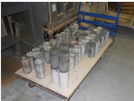
An array of concrete cylinders that are concrete samples awaiting testing. Five cylinders are created for each section of concrete. These are tested over a series of days to verify the concrete's strength and conformity with the design specifications.
