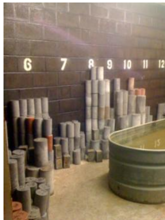
Once the samples have been poured, the concrete cylinders are placed in a special room that maintains the samples at 100% humidity.
